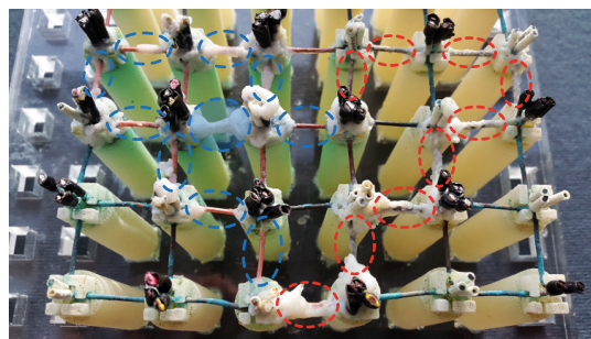
Figure 4 – Resultant heart shape growth establishes that a distributed cathode network can be used to control material properties (volume, location, composition, surface texture). 300g of marine salts were dissolved in 6.5L of water, the cathodes are 1mm copper wire, the anodes are two carbon rods of radius 6.3mm and length 75.0mm.
