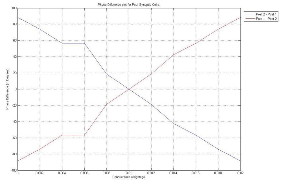
Phase difference plot for Post-Syn1 and 2 cells over a range of 0-100% strength, with step size of 10% (0.002V).
