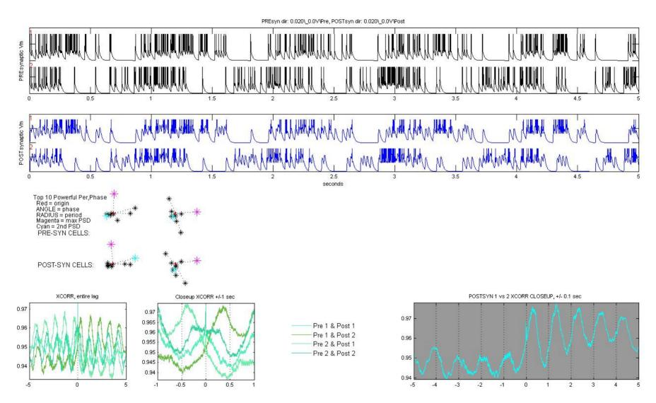
Result of the previous slide spiking network for 100% strength of Pre-Syn1 and 0% strength of Pre-Syn2 applied to Post-Syn1 and vice versa for Post-Syn2.
