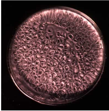
Rayleigh-Bénard convection cells in liquid heated uniformly from below (Scott Camazine, http://www.scottcamazine.com )
